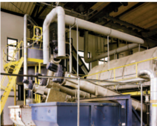
Pulper and drum screen (source: Strabag 2013)
